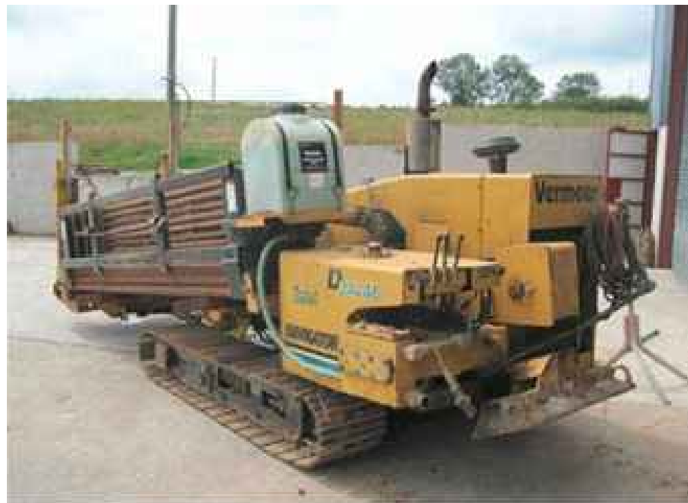
Typical Directional Drilling Rig
