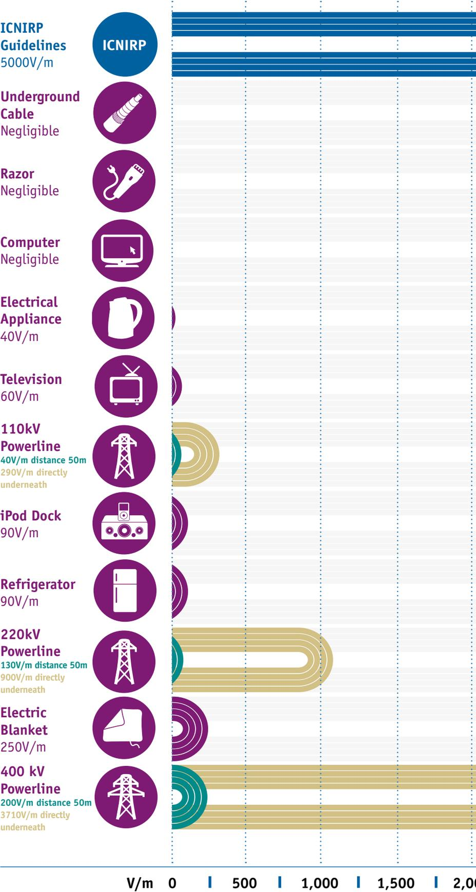
5kV/m is a reference value, 9.2kV/m is maximum allowable electric field as per the ICNIRP recommendation
