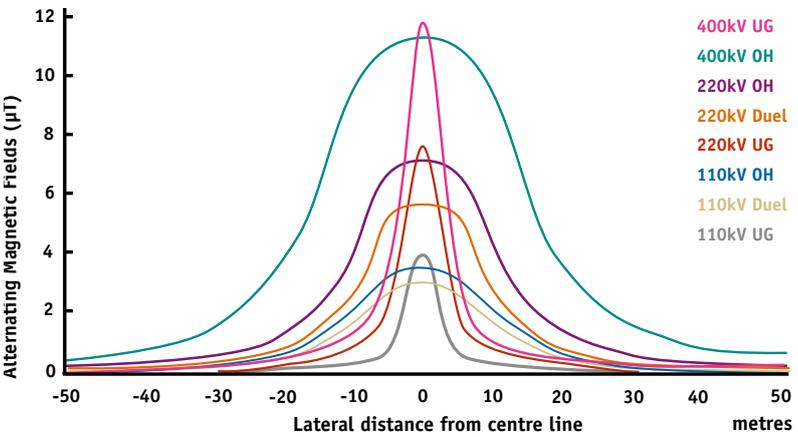
**Figure C** illustrates the magnetic field from overhead AC lines operating in Ireland. The fields strength decreases with distance. The fields from these AC lines are far below the 1998 ICNIRP Guidelines for exposure to AC magnetic fields (100µT). In 2010 ICNIRP updated its ELF-EMF guidelines, which included the recommendation for a 200µT reference level for exposure for the general public, but these have not yet been adopted by the European Union.
