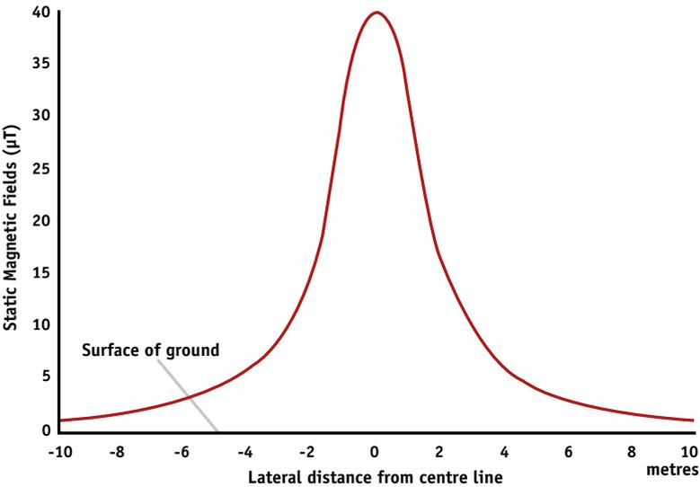
**Figure D** illustrates that the DC magnetic field decreases rapidly as you move away from the cable centre line. At a distance of 10 metres, the static magnetic field from the cable diminishes to 0.6µT. The DC magnetic field from this cable is far below the ICNIRP guideline (400,000µT).
